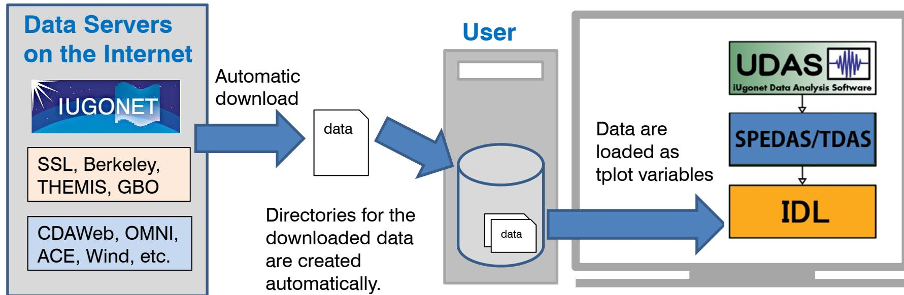
Data can be easily plotted, for example, by only three basis commands with the SPEDAS-CUI tool.
